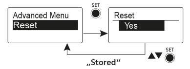
When you reset the plug-on transmitter, only the selected settings of the pilot tone and the **U** frequency bank are retained.
