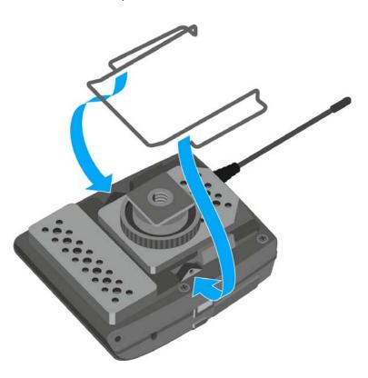
Slide the receiver onto a camera.
