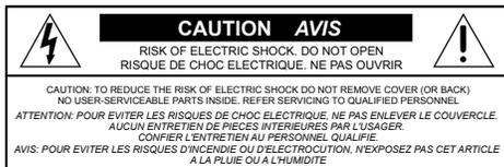
The lightning flash with arrowhead symbol within an equilateral triangle is intended to alert the user to the presence of uninsulated "dangerous voltage" within the product's enclosure, that may be of sufficient magnitude to constitute a risk of electric shock to persons.
