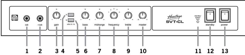
**12. STANDBY SWITCH:** Use this switch to turn the standby power on or off. Press the top of the switch to turn the standby on. The Standby mode allows the tubes to warm or remain warm without high voltage being applied to them. This extends tube life. This switch should be OFF when first turning the amplifier on. Allow the unit to warm up for at least 20 seconds before switching to the ON position. During short periods of non-use, the amp should be put into Standby mode.
