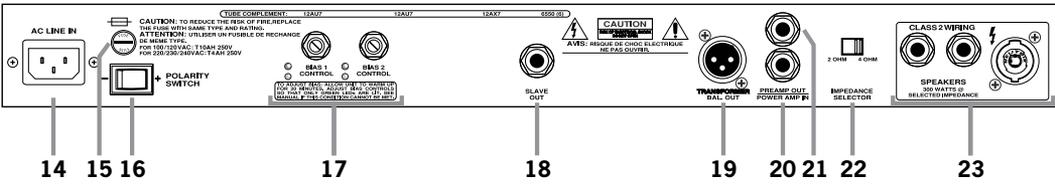
**16. POLARITY:** Place this switch in the position that provides the least electrical buzz from the unit.
