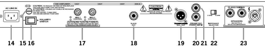
**14. IEC POWER INPUT CONNECTOR:** This is where you connect the supplied AC power cord. Plug the male end of the cord into a grounded AC outlet. **DO NOT DEFEAT THE GROUND PRONG OF THE AC PLUG!**
