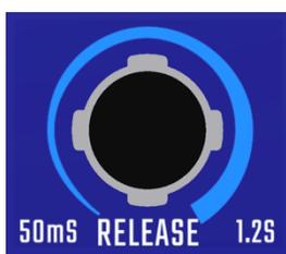
**RELEASE:** Sets the time it takes the compressor to recover to unity gain after levels fall below the set **THRESHOLD**
