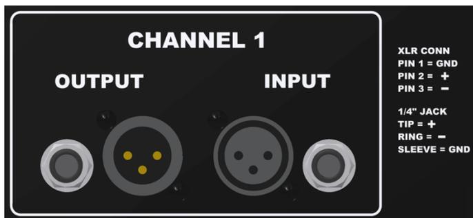
*IMPORTANT NOTE: The XLR and 1/4" INPUT connectors are wired together, so use only one INPUT connection a time.*
