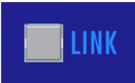
**LINK:** Toggle to link channels 1 and 2 for stereo operation
