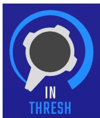
**IN THRESH** (Input/Threshold): Sets the input level/threshold
